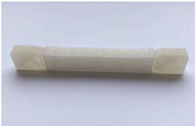
PCU test part made of various shore hardnesses
